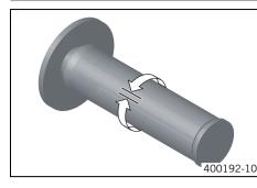
Move the handlebar to the straight-ahead position. Move the throttle grip backwards and forwards to ascertain the play in the throttle cable.
