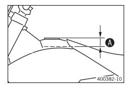
– Fill the fuel tank with fuel up to measurement  $\boldsymbol{\Theta}$ .
