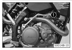
The kick starter ① is fitted on the right of the engine. The engine can be started with either the kick starter or the electric starter. The upper part of the kick starter can be swung out.
