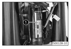
The type label **1** is fixed to the front of the steering head.
