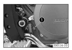
Remove gear oil level check screw 1.
