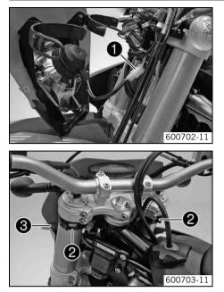
Connect the electric plug connector ①.
