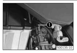
Choke ● is fitted on the left side of the carburetor. Activating the choke function frees an opening through which the engine can draw extra fuel. This gives a richer fuel-air mixture, which is needed for a cold start.
