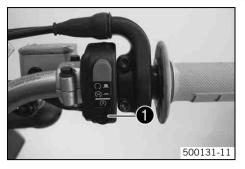
The electric starter button  ${\ensuremath{\textcircled{}}}$  is fitted on the right side of the handlebar.
