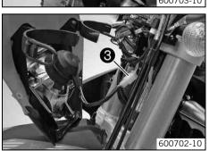
Pull out the electric plug connector ③ and remove the headlight mask with the headlight.
