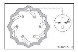
Check the thickness of the front and rear brake discs at several places on the disk to see if it conforms to measurement **(3**).
