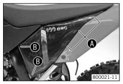
Insert the air filter box lid into the rear area  $oldsymbol{0}$  and clip it into the front area  $oldsymbol{0}$ .
