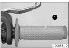
The throttle grip  $\bullet$  is fitted on the right side of the handlebar.
