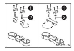
Remove the four screws **1**. Remove the handlebar clamps. Remove the handlebar and lay it to one side.
