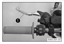
The clutch lever **1** is fitted on the left side of the handlebar. The clutch is hydraulically operated and self-adjusting.
