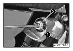
Turn adjusting screw **1** clockwise with a screwdriver up to the last perceptible click.
