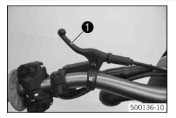
The choke lever ① is fitted on the left side of the handlebar. Activating the choke function frees an opening through which the engine can draw extra fuel. This gives a richer fuel-air mixture, which is needed for a cold start.
