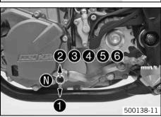
The gear positions can be seen in the photograph. The neutral or idle position is between the first and second gears.
