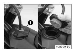
Press release button **1**, turn filler cap counterclockwise and lift it upwards and remove.
