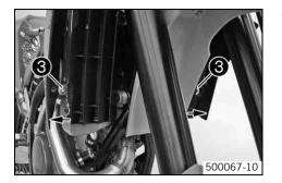
Pull both spoilers to the side of the radiator bracket ③ and take the fuel tank away upward.
