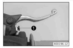
Check the free travel of the hand brake lever. (♥ p. 64) Adjust the basic setting of the hand brake lever to your hand size by turning adjusting screw ●.
