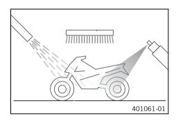
Close off the exhaust system to prevent water from entering.
