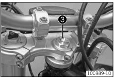
Clean the bearing and sealing elements, check for damage, and grease. \_
