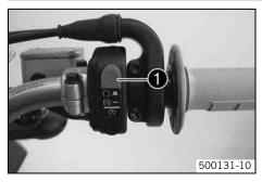
The light switch **①** is fitted on the left side of the handlebar.
