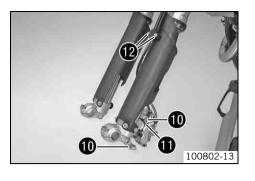
Position the brake caliper. Mount and tighten screws **(0**.
