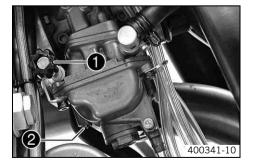
The idle setting of the carburetor has a big influence on the starting behavior, stable idling and the response to throttle opening. That means that an engine with a correctly set idle speed is easier to start than if the idle is set wrongly.
