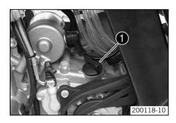
Remove the screw cap **1** and fill up with gear oil.
