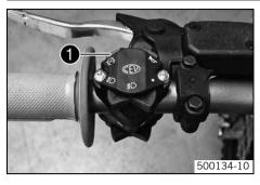
The short circuit button **1** is fitted on the left side of the handlebar.
