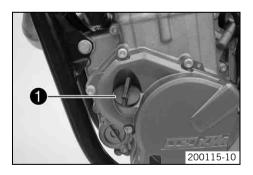
Remove the screw cap **1** on the alternator cover and fill up with engine oil.
