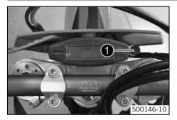
The light switch **1** is on the right of the speedometer.
