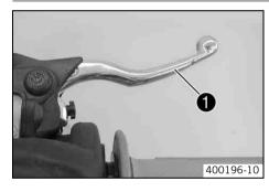
Hand brake lever  $\bullet$  is located on the right side of the handlebar. The hand brake lever is used to activate the front brake.
