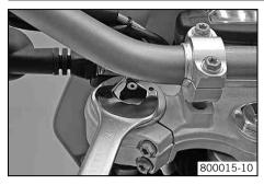
Turn the adjusting screws counterclockwise until they stop.
