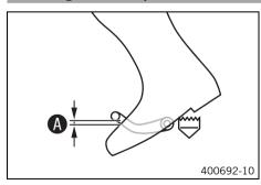
Sit on the vehicle in the riding position and determine the distance (a) between the upper edge of your boot and the shift lever.
