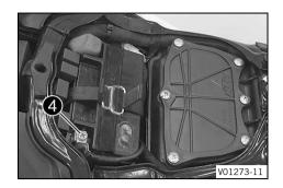
Position negative cable 4; mount and tighten the screw.
