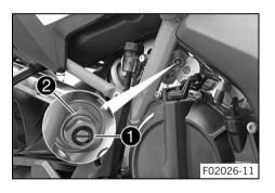
Turn adjusting screw 1 all the way clockwise with a socket wrench.
