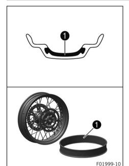
This vehicle uses a tubeless tire system in which a rim seal band 1 is used instead of the conventional tube.
