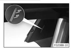
Check the coolant level in the compensating tank.
