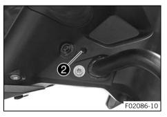
Turn adjusting screw **2** to adjust the headlight range.
