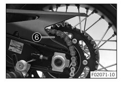
Push the rear wheel forward as far as possible. Take the chain off the rear sprocket and place it on chain sprocket guard 6.
