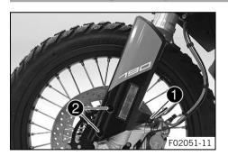
Position the fork protector. Mount screw 1, but do not tighten yet.
