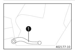
Foot brake lever **1** is located in front of the right footrest. The rear brake is activated using the foot brake lever.
