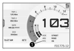
The  $\bigcirc$  area of the display indicates whether  $\underline{\mathsf{MTC}}$  ( $\bigcirc$  p. 292) is switched on or off.
