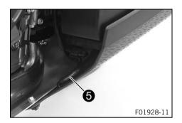
Attach tube **5** to the angle piece.
