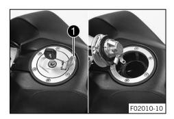
Lift cover of the fuel tank filler cap and insert the ignition key into the lock.
