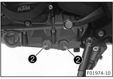
Remove oil drain plugs 2 with the magnets, O-rings, and oil screens.
