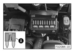
Remove the faulty fuse.
