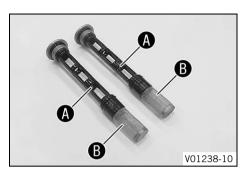
Thoroughly clean magnets **(A)** and oil screens **(B)** of the oil drain plugs.
