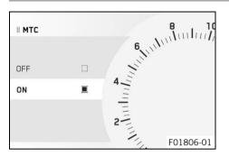
The motorcycle traction control (**MTC**) lowers the engine torque in case of loss of traction in the rear wheel.
