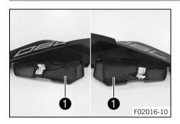
The left or right storage compartment contains the on-board tool set  $\ensuremath{\text{\textbf{1}}}$ .
