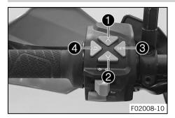
The menu switch is fitted in the middle of the left combination switch.
