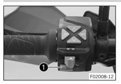
The horn button **1** is fitted on the combination switch on the left.
