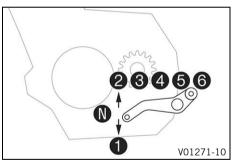
The gear positions can be seen in the figure.
