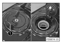
Lift cover of the fuel tank filler cap and insert the ignition key into the lock.
