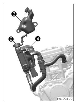
The coolant is cooled by the air stream and a radiator fan **4**, which is activated at high temperature.
