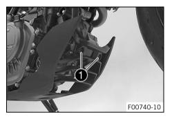
Position the front spoiler. Mount screws 1 but do not tighten yet.
