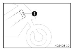
The vehicle identification number  $\P$  is stamped on the right side of the steering head.
