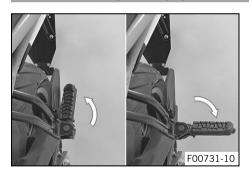
The passenger foot pegs can be folded up and down.
