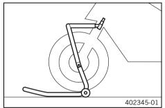
Move the handlebar to the straight-ahead position. Position the lifting gear.
