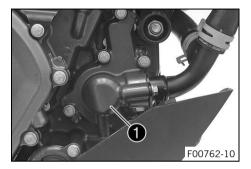
Water pump **1** in the engine ensures forced circulation of the coolant.
