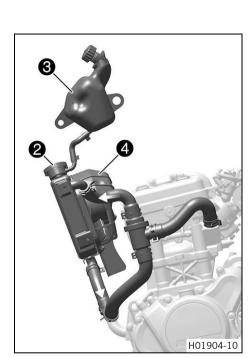
The coolant is cooled by the air stream and a radiator fan **4**, which is activated at high temperature.
