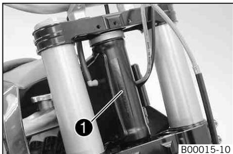
The chassis number ❶ is stamped on the right side of the steering head.
